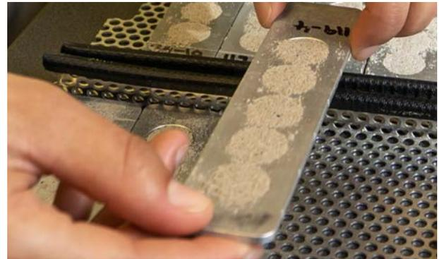
Sand Samples being Dried using RemScan's Portable Drying Unit
