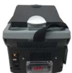
RemScan provides a warning error if samples are above 5% free moisture content, Wet soil samples can be air-dried, or dried using the Portable Drying Unit.
